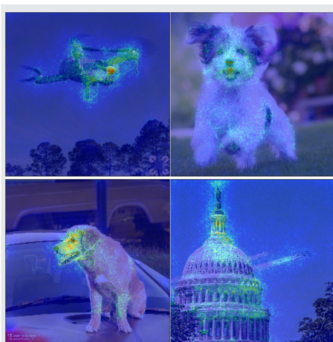
Figure 2. Saliency maps were overlaid on the 4 images. Upper left: A drone; Upper right: A dog; Bottom left: An AI generated dog; Bottom right: The Capitol Dome.
